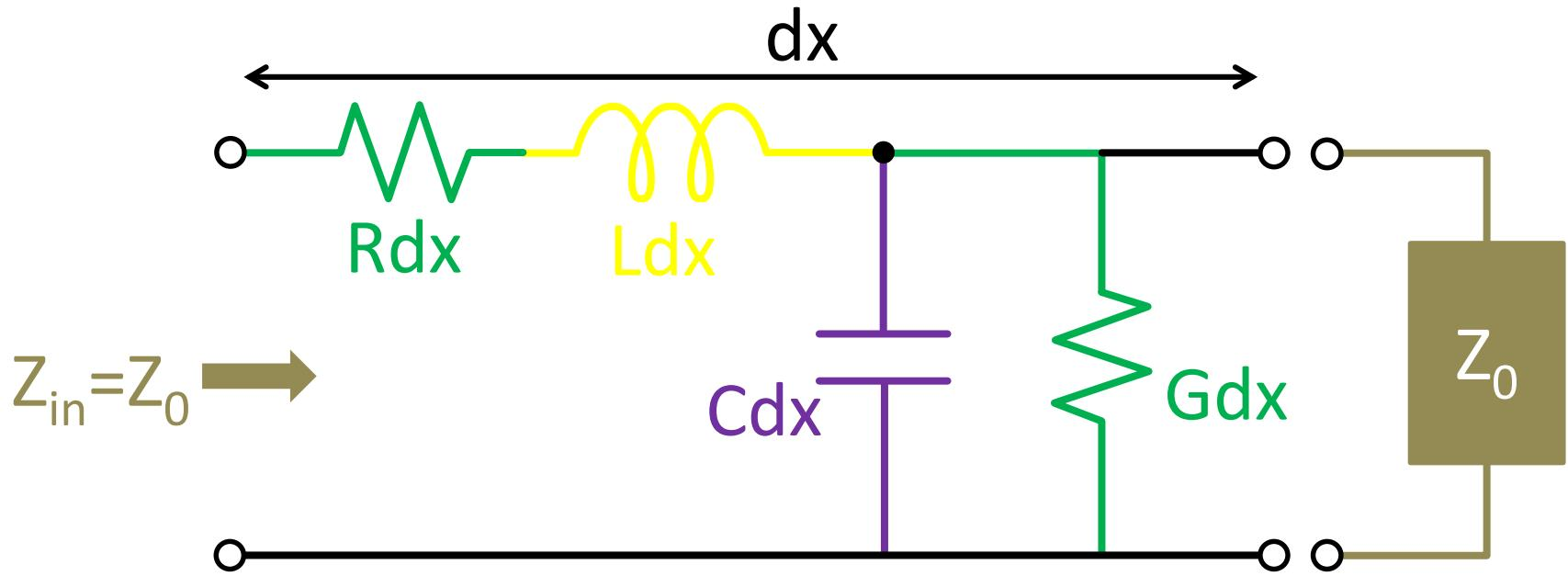
$$Z_0 = R_{dx} + j\omega L_{dx} + Z_0 \parallel \left( \frac{1}{G_{dx} + j\omega C_{dx}} \right)$$
