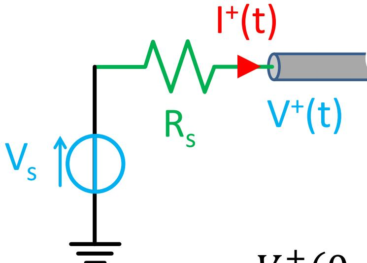
$$\begin{aligned} V_s &= V^+ + I^+ R_s \\ &= V^+ \left( 1 + \frac{R_s}{Z_0} \right) \end{aligned}$$
