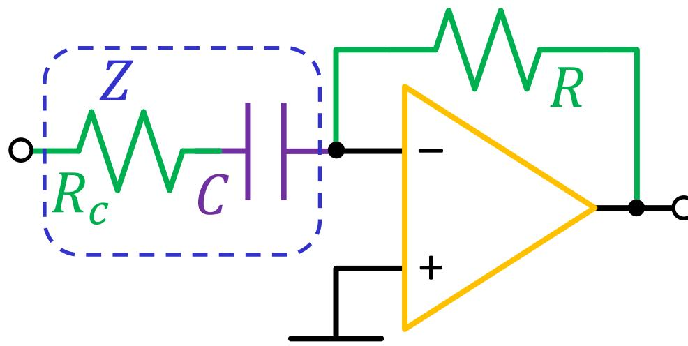
$$\begin{aligned} \frac{V_o}{V_i} &= -\frac{R}{Z} = -\frac{R}{R_c + 1/sC} \\ &= -\frac{sCR}{1 + sCR_c} \end{aligned}$$
