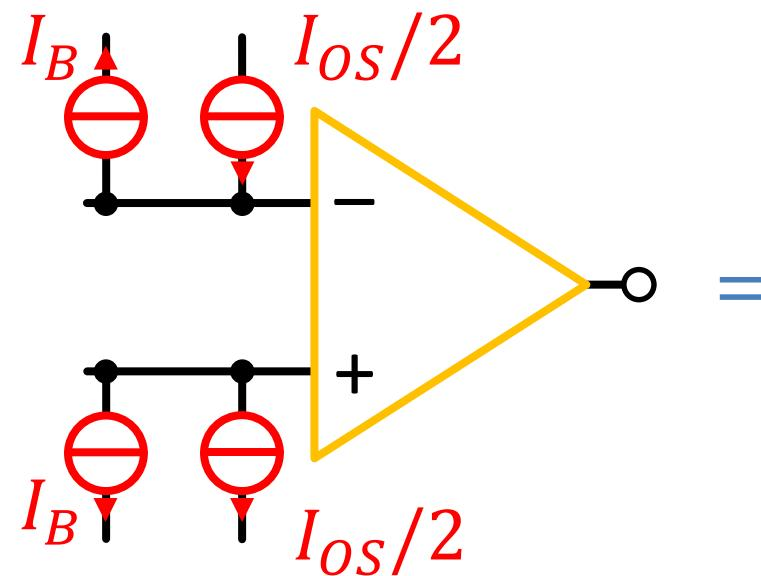
$$\left. \begin{array}{l} I_B = \frac{I_b^+ + I_b^-}{2} \\ I_{OS} = I_b^+ - I_b^- \end{array} \right\} \Rightarrow \begin{array}{l} I_b^+ = I_B + \frac{I_{OS}}{2} \\ I_b^- = I_B - \frac{I_{OS}}{2} \end{array}$$
