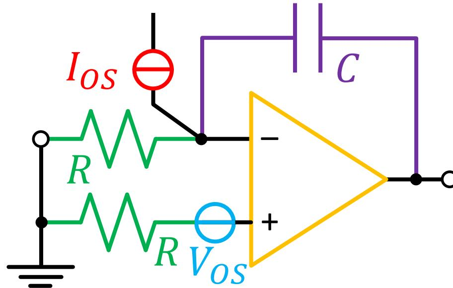
$$V_o = \frac{I_{os}}{sC} + V_{os} \left( 1 + \frac{1}{sCR} \right)$$
