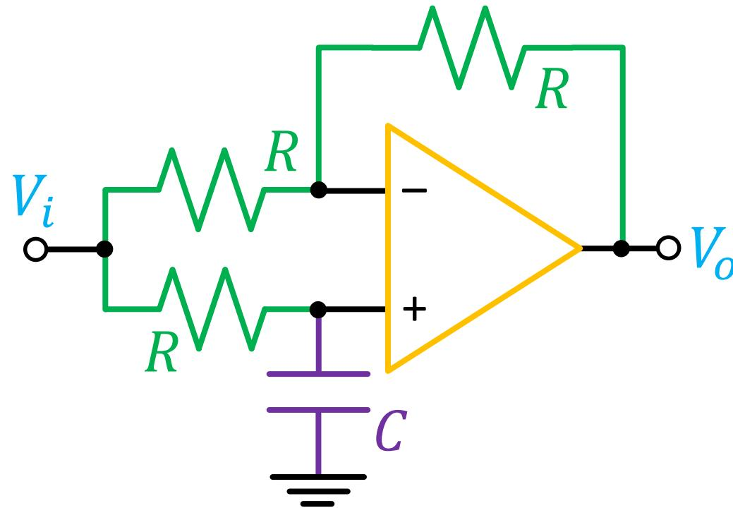
$$\begin{aligned}C &= 10 \text{ nF} \\R &= 2 \text{ k}\Omega \\\tau &= 16 \text{ ms} \\A_0 &= 10^6\end{aligned}$$
