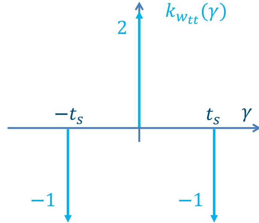
$$k_{wtt}(\gamma) = 2\delta(\gamma) - \delta(|\gamma| - t_s)$$
