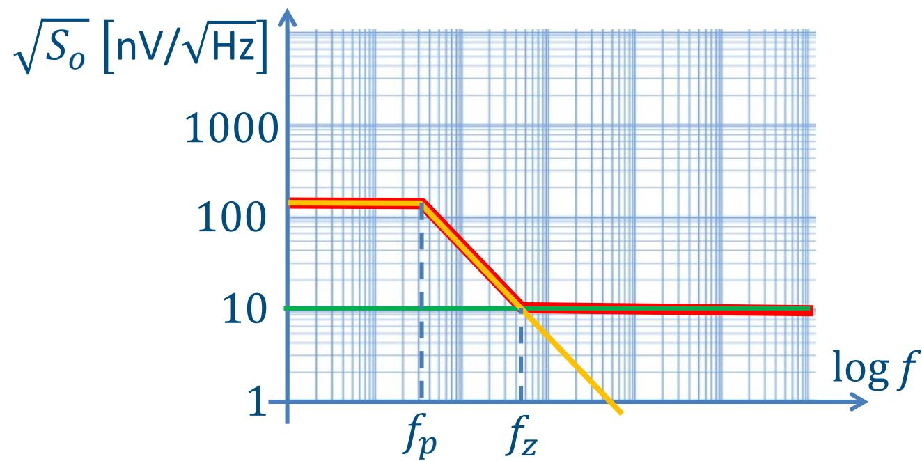
$$f_p = \frac{1}{2\pi C_S R_S} = 31.8 \text{ kHz}$$
