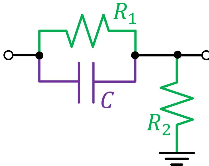
$$H_w(s) = \frac{R_2}{R_1 + R_2} \frac{1 + sCR_1}{1 + sC(R_1 \parallel R_2)} = \frac{1}{2\pi f_z} \approx 383 \text{ ns}$$
