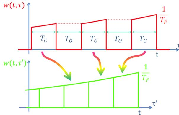
Figure 3: (Top) weighting function of the BA. (Bottom) Equivalent-time weighting function of the BA.
