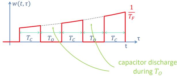
Figure 5: Weighting function of the ratemeter integrator.
